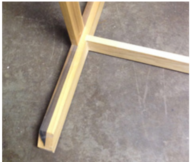
Above: image of the large frame displaying the half-lapped lattice work that secures the plexi-glass.
